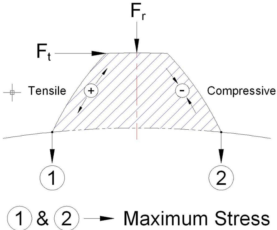
Figure 1. Tangential and Radial forces on gear tooth.
