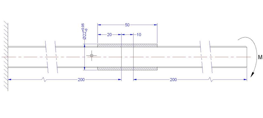
**Figure 6. Experimental setup.**
