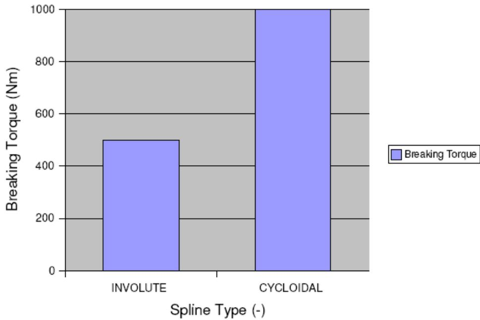
**Figure 7. Torque Capacity results from TTR testing.**
