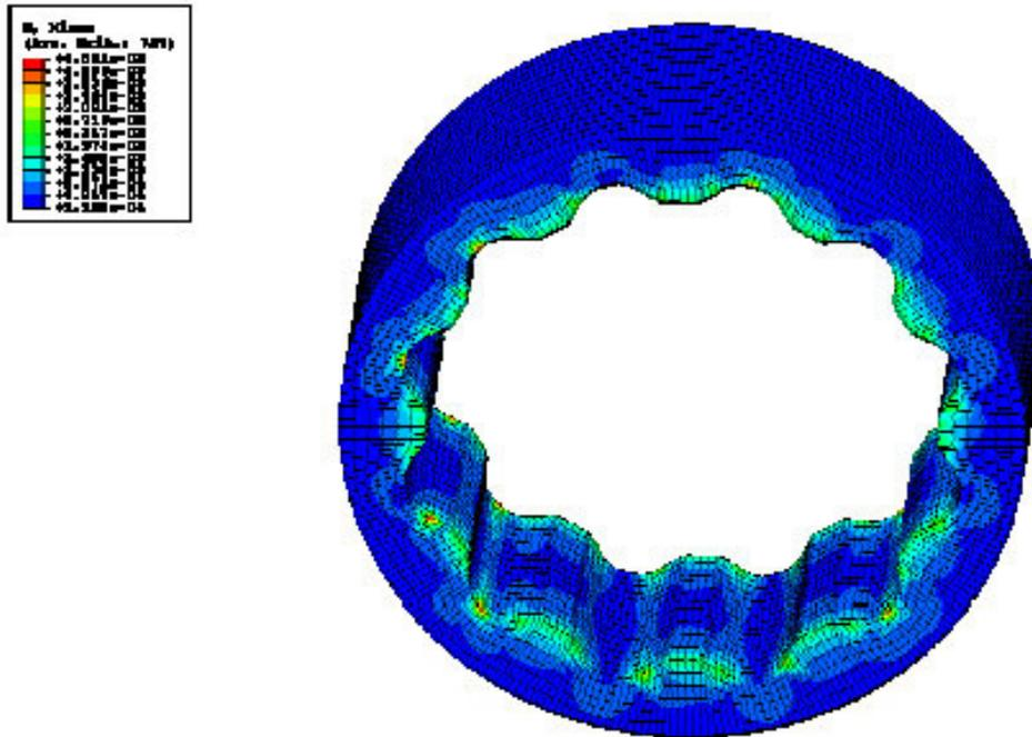
Figure 3. STEER's FEM analysis of Continua splines. (ANSYS 10)
