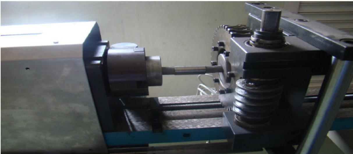
Figure 4. STEER's Torsional Test Rig.
